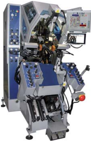
CERIM HYDRAULIC LASTING MACHINE WITH INJECTION SYSTEM PREMONTA E MONTA IDRAULICA PROGRAMMABILE
