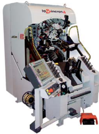
MOLINA&BIANCHI PNEUMATIC LASTING MACHINE WITH INJECTION SYSTEM PREMONTA E MONTA PNEUMATICA PROGRAMMABILE
