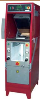
PNEUMATIC PRESS FOR STICKING THE SOLES OR TRAINER PRESSA A CAMPANA
