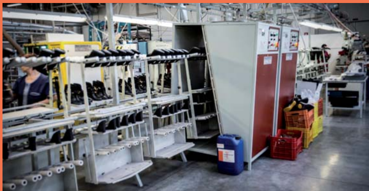
LASTING CONVEYOR MANOVIA MONTAGGIO
