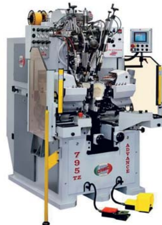
ORMAC HYDRAULIC TACK HEEL SEAT AND SIDES LASTING MACHINE WITH T.P. MONTABOETTE A CHIODI E FIANCHI TERMOPLASTICO COMPUTERIZZATA
